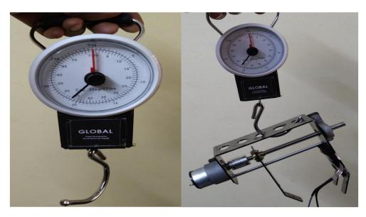
Figure 11. Analog weighing scale & gripper weight measurement
