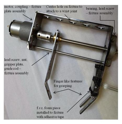
Figure 9. L.S.Gripper assembly construction
