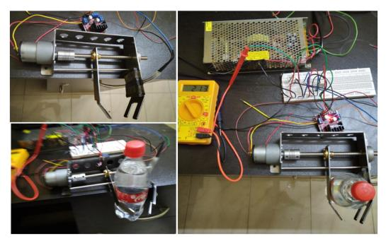
Figure 10. L.S.Gripper assembly operation
