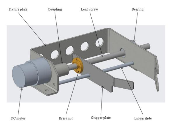
Figure 1. CAD assembly model of l.s.gripper
