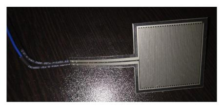
Figure 6. Force sensitive resistor, 40x40 mm area
