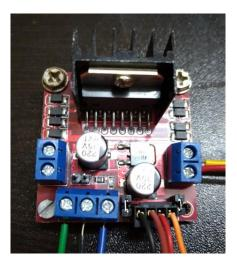
Figure 5. L298 DC motor driver board
