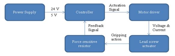
Figure 4. Mechatronic system concept for the l.s.gripper
